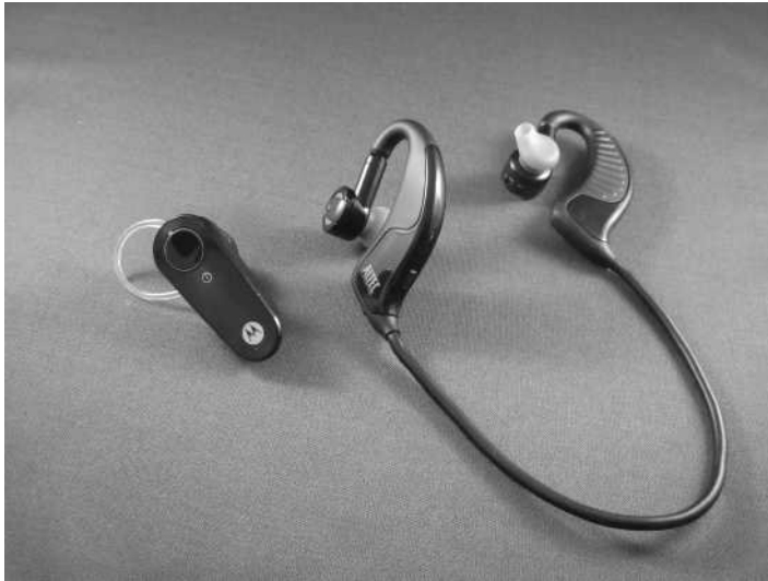
Figure 1-2 Two examples of Bluetooth headsets: mono (left) and stereo (right)
